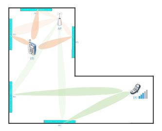
Fig. 1. A smart radio environment with multiple RISs. User A is far away from the AP and suffers from low received signal strength, while user B has amble received power but a low-rank ill-conditioned channel. The RISs can be optimized to help in both scenarios.
