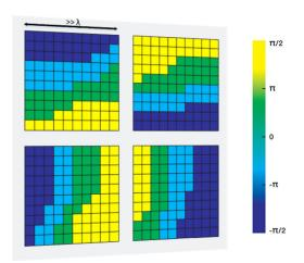
(b) A 4-element metasurface-based RIS. Each element/tile is a dynamic metasurafce with numerous tightly-packed metaatoms and can apply an arbitrary quasi-continuous phase gradient.
