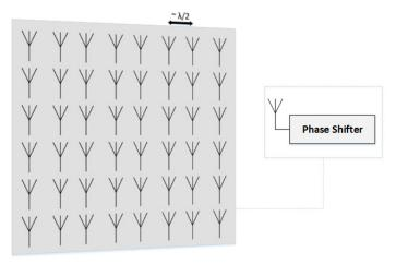
(a) A 48-element reflectarray-based RIS. Each element is a traditional antenna connected to a phase shifter.
