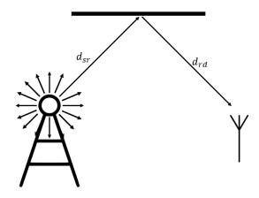
(b) Large-scale path loss of reflected electromagnetic waves.
