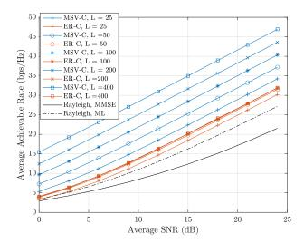
Fig. 3. The effect of the number of RIS elements, L, on the achievable rate when the phase shifts are optimized according to MSV-C and ER-C.  $\alpha = 0.5$  for all curves. The achievable rate of the canonical Rayleigh channel is also shown for the ML and MMSE receivers as baselines.
