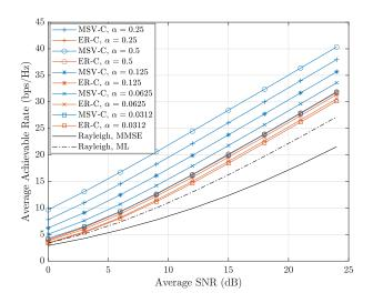
Fig. 4. The effects of the power fraction,  $\alpha$ , on the achievable rate when the phase shifts are optimized according to MSV-C and ER-C. L = 100 for all curves. The achievable rate of the canonical Rayleigh channel is also shown for the ML and MMSE receivers as baselines.
