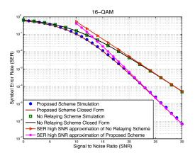
Fig. 3. The symbol error rate (SER) for the 16-QAM constellation.
