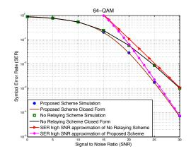
Fig. 4. The symbol error rate (SER) for the 64-QAM constellation.
