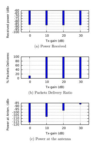
Figure 5: From top to bottom power received, packet delivery ratio and estimated power at the antenna when the sum of tx-gain and rx-gain is held constant at 30 dB.
