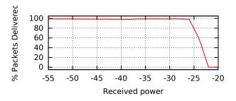
Figure 3: Saturation occurs when the power received is too high. BPSK modulation was used.
