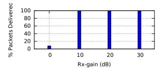
Figure 4: The effect of changing the rx-gain on packet delivery when tx-gain is constant.
