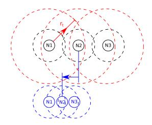
Figure 1: To test a relay scenario, starting from nodes displayed with black, the user can change gains as shown in red, or change the placement of nodes shown in blue. Dashed circles present the transmission range.
