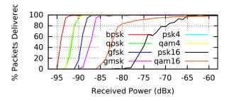
Figure 2: Relation between the received power and the packet delivery ratio for different types of modulation.
