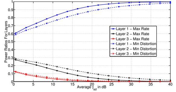
Fig. 2: The optimal power ratios of the layers versus  $\bar{\gamma}$  for three layers transmitted over a Rayleigh fading AF relay channel with  $(m_1, m_2) = (16, 16)$ .
