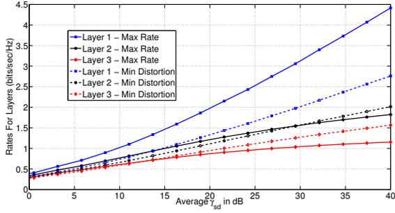
Fig. 3: The optimal rates of the layers versus  $\bar{\gamma}$  for three layers transmitted over a Rayleigh fading AF relay channel with  $(m_1, m_2) = (16, 16)$ .
