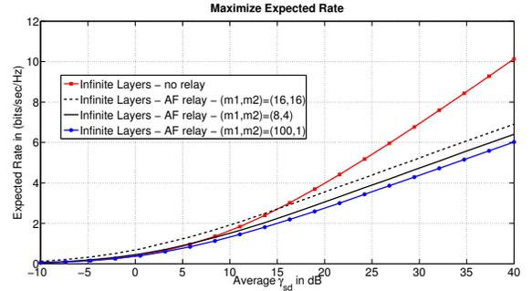
Fig. 6: The expected sum rate versus  $\bar{\gamma}$  with infinite number of layers transmitted over a Rayleigh fading channel with and without using a relay with the objective of maximizing the expected sum rate.
