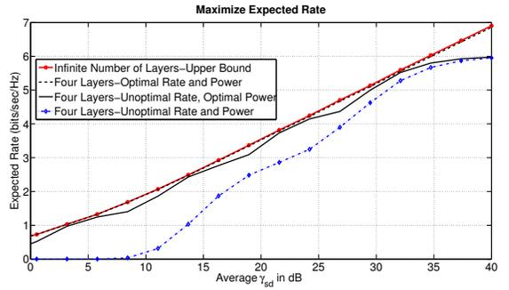
Fig. 5: The expected sum rate versus  $\bar{\gamma}$  over a Rayleigh fading AF relay channel with  $(m_1, m_2) = (16, 16)$  with the objective of maximizing the expected sum rate.
