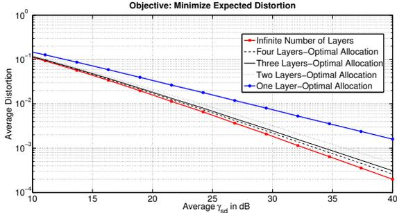
Fig. 4: The average distortion versus  $\bar{\gamma}$  for various number of layers transmitted over a Rayleigh fading AF relay channel with  $(m_1, m_2) = (16, 16)$  with the objective of minimizing the average distortion.
