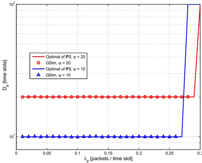
Fig. 5. The delay-throughput tradeoff at the PU,  $\lambda_s = 0.2$ . The corresponding PU delay of the BL takes arbitrarily large values [13] and, hence, it is not plotted. The parameters of the wireless channel are  $h_{pd} = 0.3$ ,  $h_{ps} = 0.4$ , and  $h_{sd} = 0.8$ .
