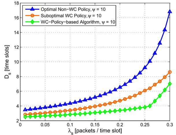
Fig. 6. The average delay of the SU packets versus the arrival rate of the SU packets under different cooperation policies,  $\lambda_p = 0.2$  and  $\psi = 10$ . The parameters of the wireless channel are  $h_{pd} = 0.3$ ,  $h_{ps} = 0.4$ , and  $h_{sd} = 0.8$ .
