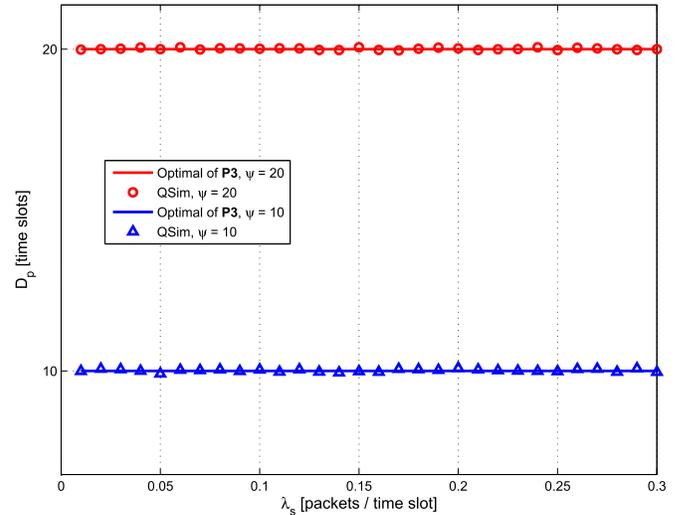
Fig. 4. The average PU packet delay versus the arrival rate of the SU packets,  $\lambda_p = 0.2$ . The corresponding PU delay of the BL takes arbitrarily large values [13] and, hence, it is not plotted. The parameters of the wireless channel are  $h_{pd} = 0.3$ ,  $h_{ps} = 0.4$ , and  $h_{sd} = 0.8$ .
