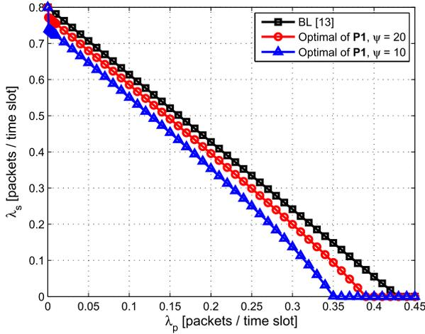
Fig. 2. The stable throughput region. The parameters of the wireless channel are  $h_{pd} = 0.3$ ,  $h_{ps} = 0.4$ , and  $h_{sd} = 0.8$ .
