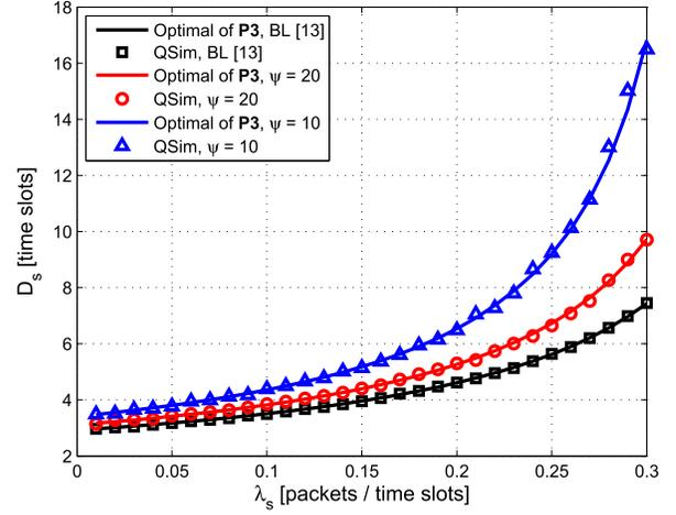
Fig. 3. The delay-throughput tradeoff at the SU,  $\lambda_p = 0.2$ . The parameters of the wireless channel are  $h_{pd} = 0.3$ ,  $h_{ps} = 0.4$ , and  $h_{sd} = 0.8$ .
