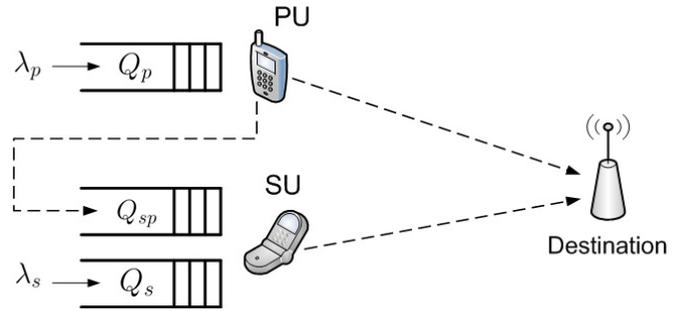
Fig. 1. The system model. The dashed lines represent communication links between nodes.
