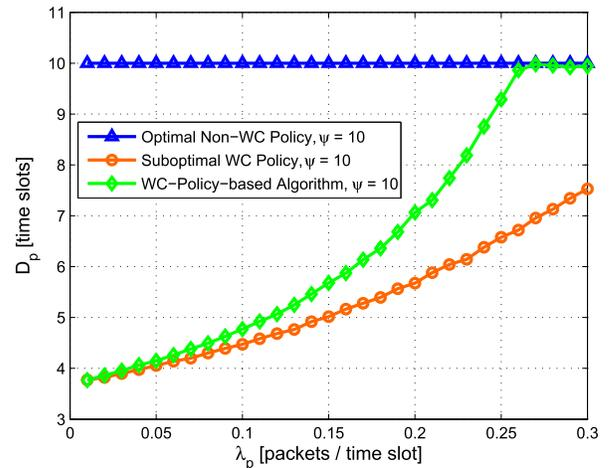
Fig. 7. The average delay of the PU packets versus the arrival rate of the SU packets under different cooperation policies,  $\lambda_p = 0.2$  and  $\psi = 10$ . The parameters of the wireless channel are  $h_{pd} = 0.3$ ,  $h_{ps} = 0.4$ , and  $h_{sd} = 0.8$ .
