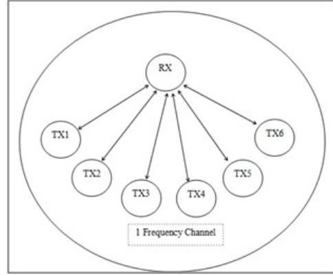
Fig. 2: The Native Topology of the NRF24L01+ Module
