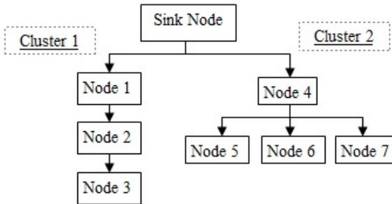
Fig. 4: The Network Topology of Tests 1 and 2
