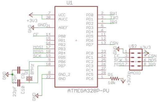
Fig. 1: The Final Hardware Design of the WSN Node
