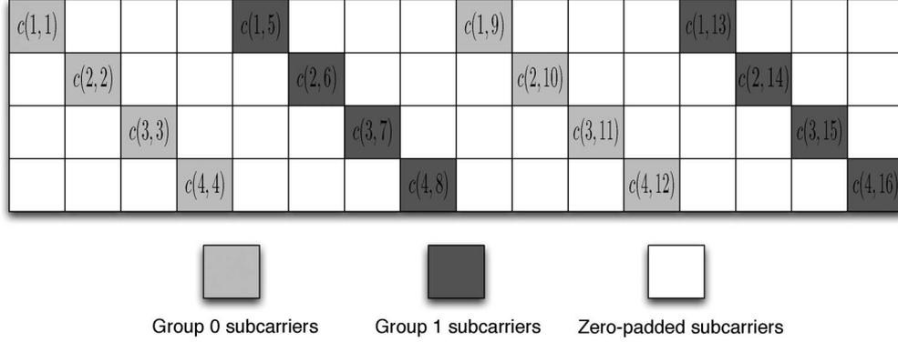
Fig. 2. Structure of code matrix  $\mathbf{C}_r$  defined in (4) for a special case of two groups, four relays, two channel taps, and 16 subcarriers.
