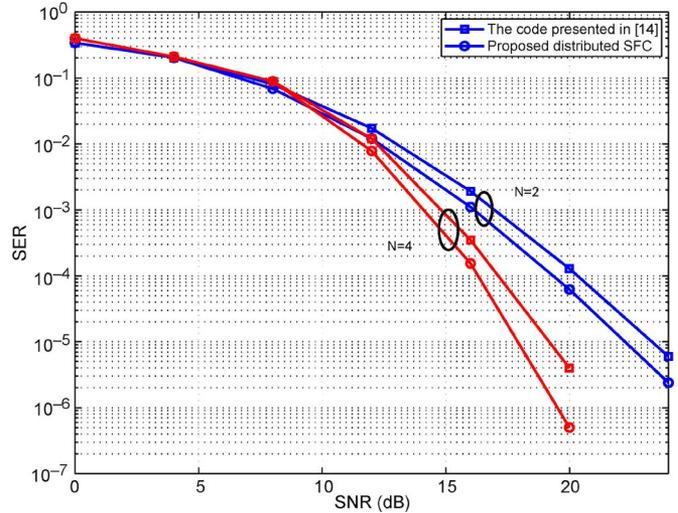
Fig. 4. Performance comparison between the proposed distributed SFC and the code proposed in [14] with different numbers of relay nodes and BPSK modulation.
