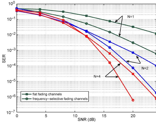
Fig. 3. SER versus SNR over both frequency-selective fading channels and flat-fading channels with one, two, and four relays. BPSK modulation is used. The delay vector  $[0, 0.5] \mu\text{s}$  is used for both the source-to-relay and relay-to-destination channels.
