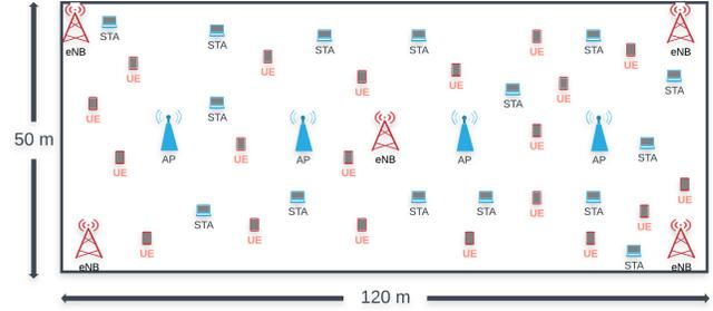
Fig. 4: Snapshot of the  $C/L$  layout of 5 eNBs located at the corners and 4 WiFi APs placed along the same line.
