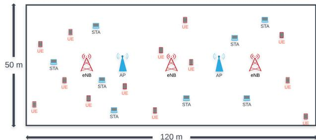
Fig. 1: Snapshot of the  $L/L$  layout of 3 eNBs and 2 WiFi APs placed along the same line.
