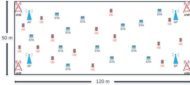
Fig. 2: Snapshot of the  $C/C$  layout of 4 eNBs and 4 WiFi APs placed at the corners.
