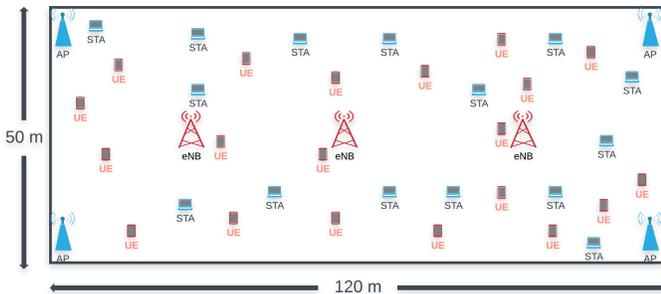
Fig. 3: Snapshot of the  $L/C$  layout of 3 eNBs placed along the same line and 4 WiFi APs placed at the corners.
