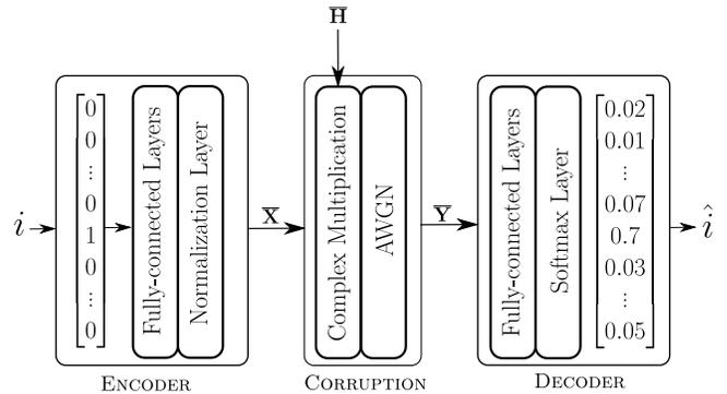
Fig. 2. Denoising autoencoder structure used for generation of noncoherent codes.
