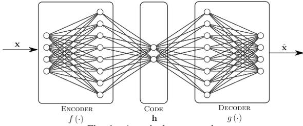
Fig. 1. A typical autoencoder.
