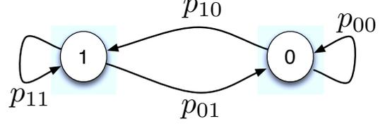
Fig. 2: Markov chain model of the PU activity
