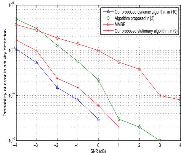
Fig. 3: The probability of error in PU activity detection for the different spatial spectrum holes detection algorithms.
