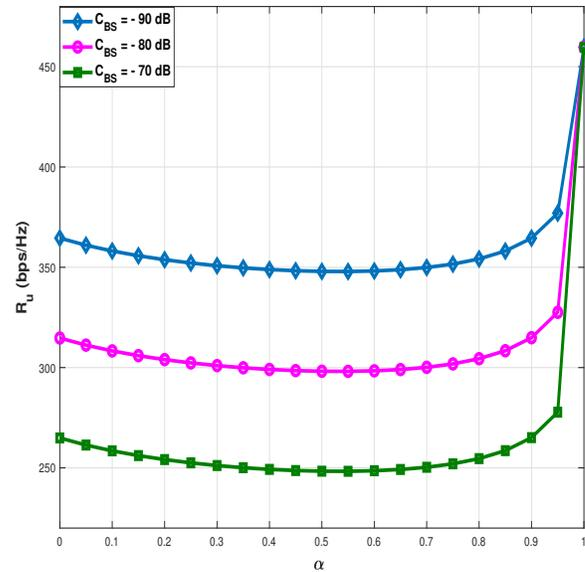
Fig. 5: Validating rate maximization problem solution when fixing  $R_d = R$  and maximizing  $R_u$ . Parameters used to generate this figure:  $N = 200$ ,  $K_d = 20$ ,  $K_u = 15$ ,  $\sigma^2 = -110dB$ ,  $R_d = R = 200bps/Hz$ ,  $P_d = 10W$  and  $P_u = 2mW$ .
