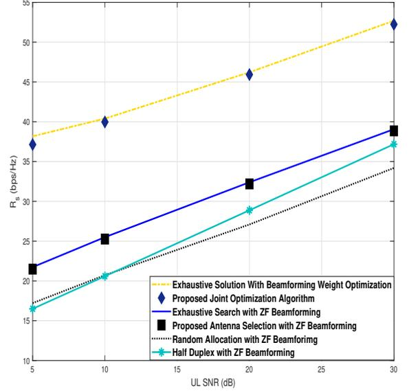
Fig. 3: Variation of the sum rate with the UL SNR for different antennas' selection algorithms in a FD network.
