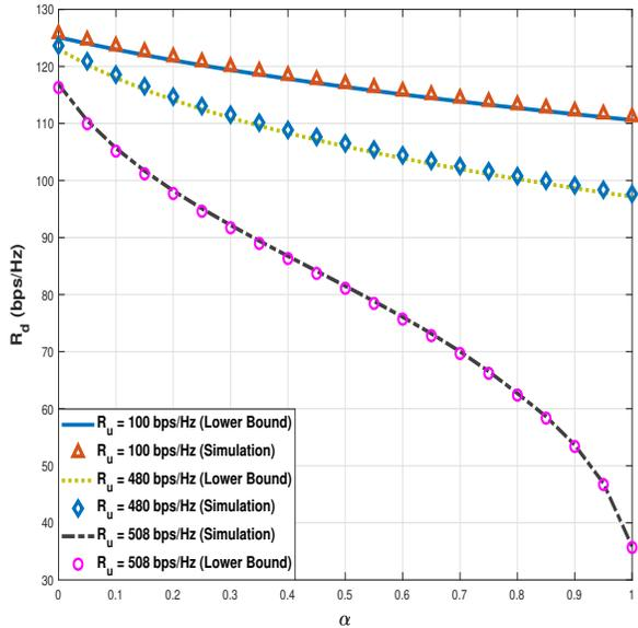
Fig. 6: Validating rate maximization problem solution when fixing  $R_u$  and maximizing  $R_d$ . Parameters used to generate This figure:  $N = 200$ ,  $K_d = 10$ ,  $K_u = 15$ ,  $\sigma^2 = -110\text{dB}$ ,  $P_d = 10\text{W}$  and  $P_u = 2\text{mW}$ , for  $R_u = 100, 480, 508\text{bps/Hz}$ .
