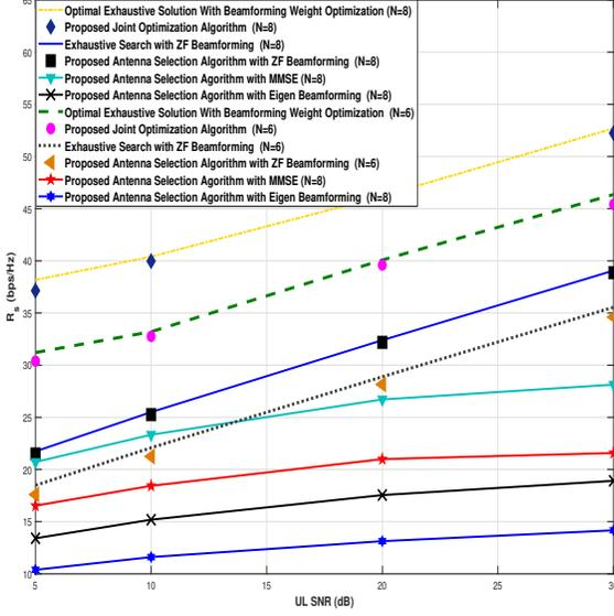
Fig. 2: Variation of the sum rate with the UL SNR for  $N = 6$ ,  $K_d = 3$ , and  $K_u = 2$  and  $N = 8$ ,  $K_d = 3$ , and  $K_u = 2$ .
