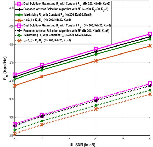
Fig. 7: Variation of the sum rate with The UL-SNR in a massive MIMO network.
