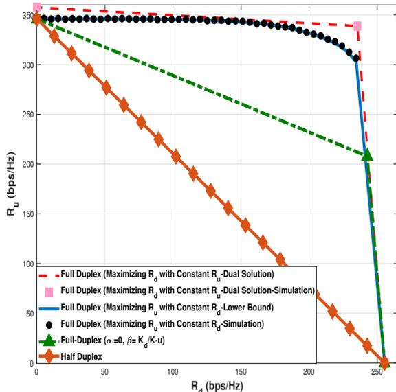
Fig. 8: Feasible rate region for different full duplex and half duplex systems. Parameters used to generate this figure:  $N = 300$ ,  $K_d = 20$ ,  $K_u = 10$ ,  $\sigma^2 = -110dB$ ,  $P_d = 10W$  and  $P_u = 2mW$ .
