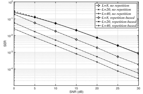
Fig. 3: SER of the QPSK modulated IRS data for  $L = 8$ ,  $L = 20$ , and  $L = 40$  with  $M = N = 2$ ; the results are shown for the no-repetition and repetition-based schemes
