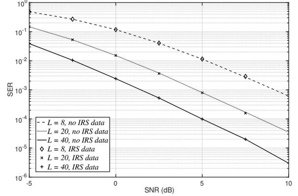
Fig. 2: SER of the schemes with IRS data transmissions and no IRS data transmission for  $L = 8$ ,  $L = 20$ , and  $L = 40$  with  $M = N = 2$  (in the legends, no IRS data means that the IRS merely reflects the transmitter impinging energy; IRS data means that some IRS elements transmit extra data symbols by controlling their phases)
