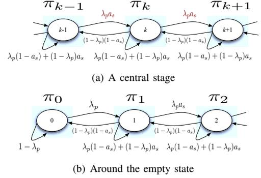
Fig. 1. The conventional PU queue evolution Markov chain
