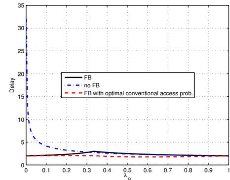
Fig. 5. The PU delay for the different access schemes.
