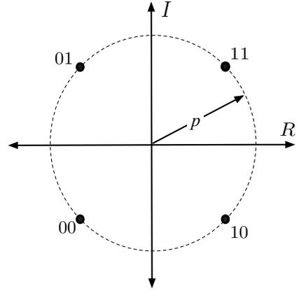
Fig. 3: QPSK signal constellation in each direction.
