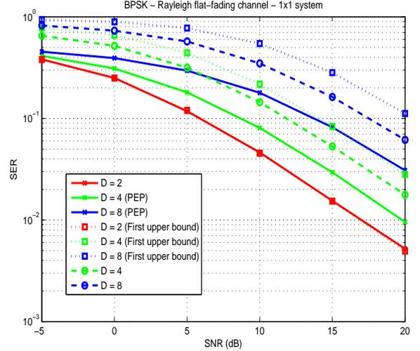
Fig. 5: Pairwise error probability and the first upper bound to the pairwise error probability curves for  $D = 2, 4$  and  $8$ .
