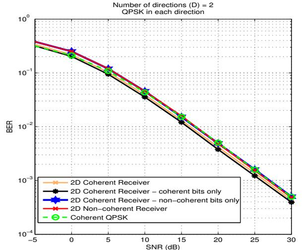
Fig. 6: Performance Curves for the coherent and non-coherent receivers in case of two directions  $D = 2$ .
