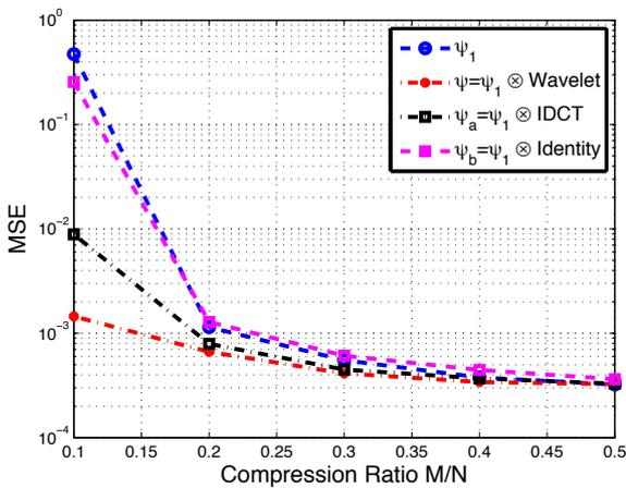
Fig. 4. MSE versus Compression Ratio under different sparsifying bases
