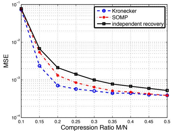
Fig. 2. MSE performance versus Compression Ratio under different recovery algorithms
