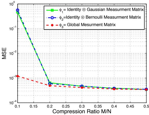
Fig. 3. MSE versus Compression Ratio using different measurements matrices
