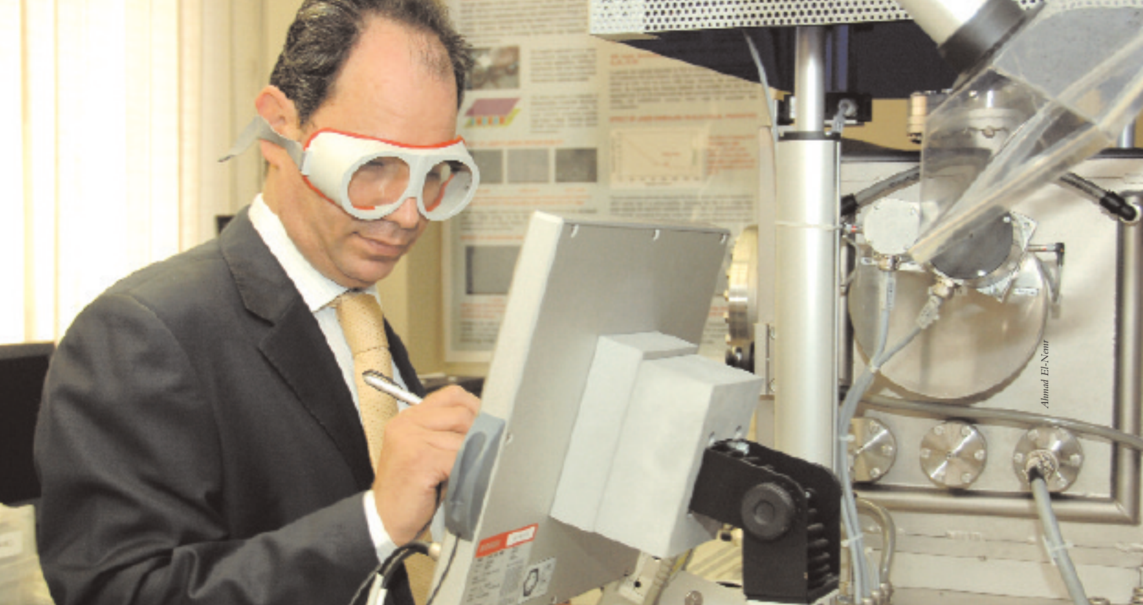
Abdel Rahman monitors the work of a pulsed laser deposition system as it prepares the alloys used to store hydrogen
